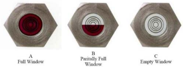
Figure 5. Oil Level Sight Glass Conditions
